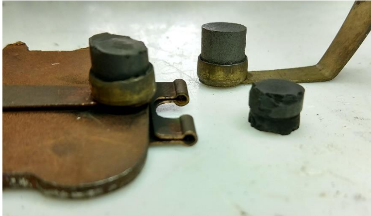
Figure 1: Old and New Carbon Brushes
