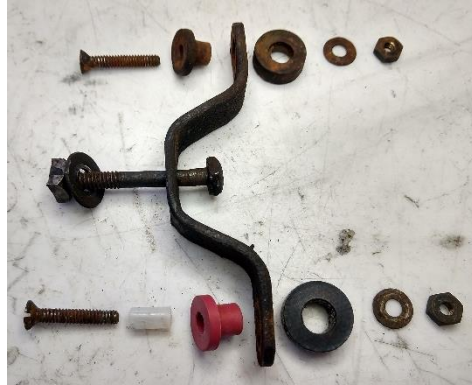
Figure 5: Signal Bell Insulation System, Old (top) and New (bottom)
