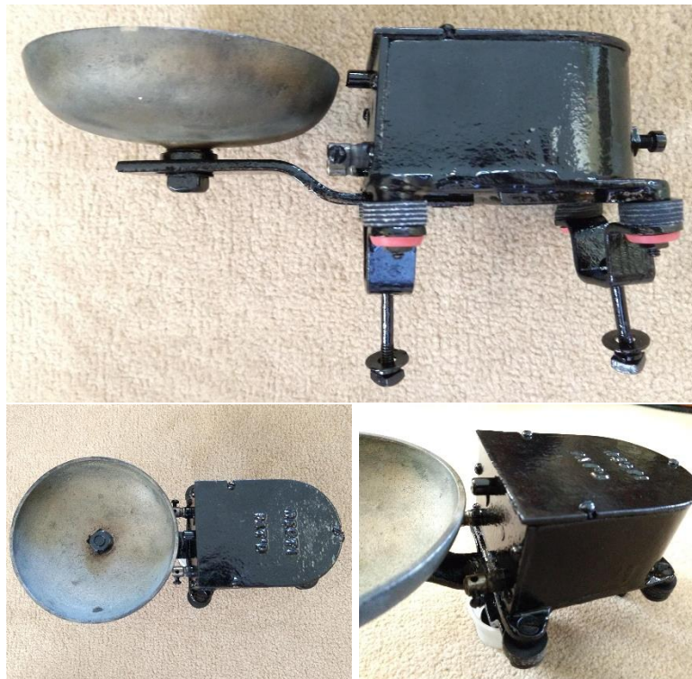
Figure 6: Painted and Assembled Signal Bell
